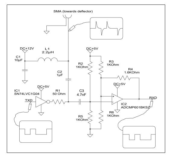
The data towards the deflector (TXD) is high pass filtered while the power supply (DC+12V) is low pass filtered. The high pass filtering is achieved through inductor L1 and resistor R1. Capacitor C2 only serves as a DC level shifter between output amplifier (IC1) and the deflector's power supply. The time constant of the high pass filter equals 44 nsec ( $2.2\mu$ H/50Ohm). The saturation current of inductor L1 should be high enough to handle the deflector's peak currents.
