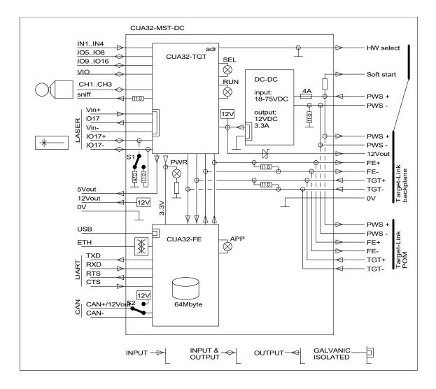
The CUA32-FE module is connected to the CUA32-TGT module using a serial bus. This Target-Link is implemented like a
