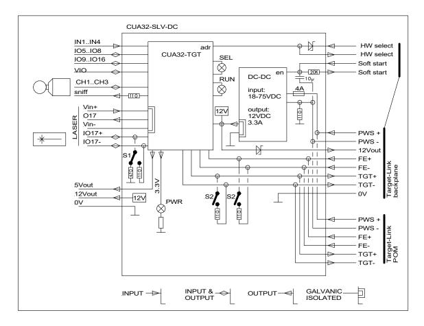
CUA32-SLV DC devices don't have a power supply connector. They are powered over the backplane or over the POM connector. Up to seven CUA32-SLV-DC devices can be attached to this backplane. To limit inrush current when powered
