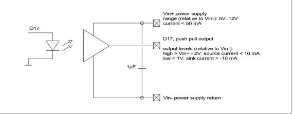
When the laser gate has TTL like interfacing, the galvanically isolated O17 output could be used. Powered by a 5V power supply (Vin+/Vin-), the O17 high level will be above 3V and the low will be below 0.3 V.
