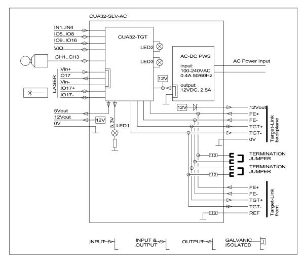
The target link is a 10 Mbit/sec serial connection. The termination jumpers should be installed on the slave device that is furthest away from the master device (CUA32-MSTR-AC).
